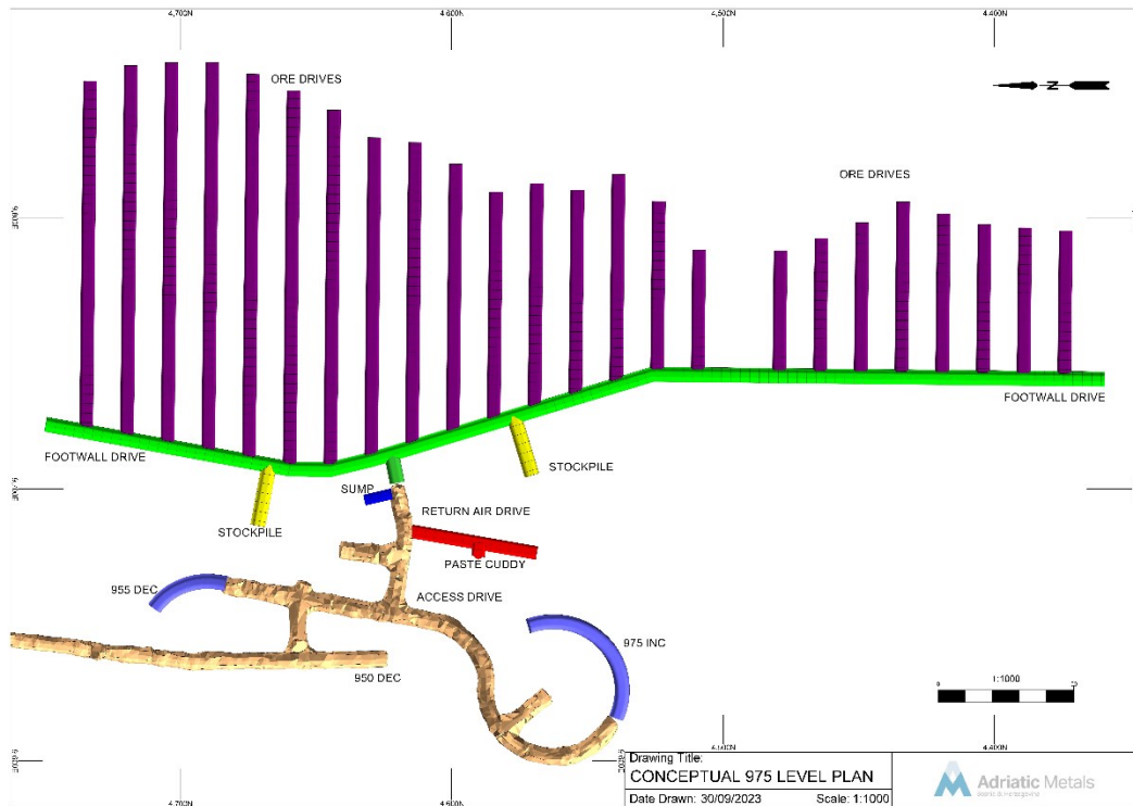
Figure 3: Rupice 975 production level plan Brown lines are development as at 10 October 2023, and purple lines are future ore drives
