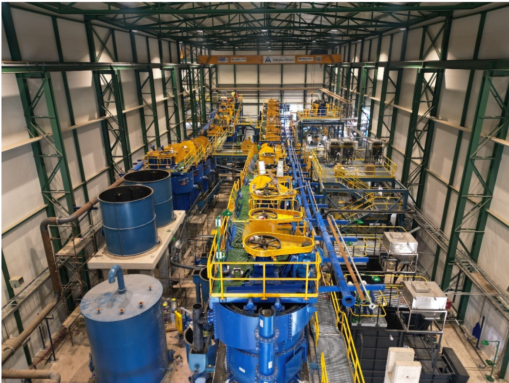
Figure 8: Looking south in zinc flotation circuit, September 2023
