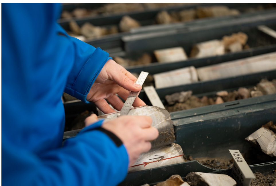
Figure 13: Core being prepared for sampling.
