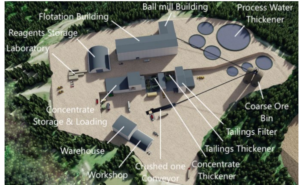
Schematic of the Vares Processing Plant
