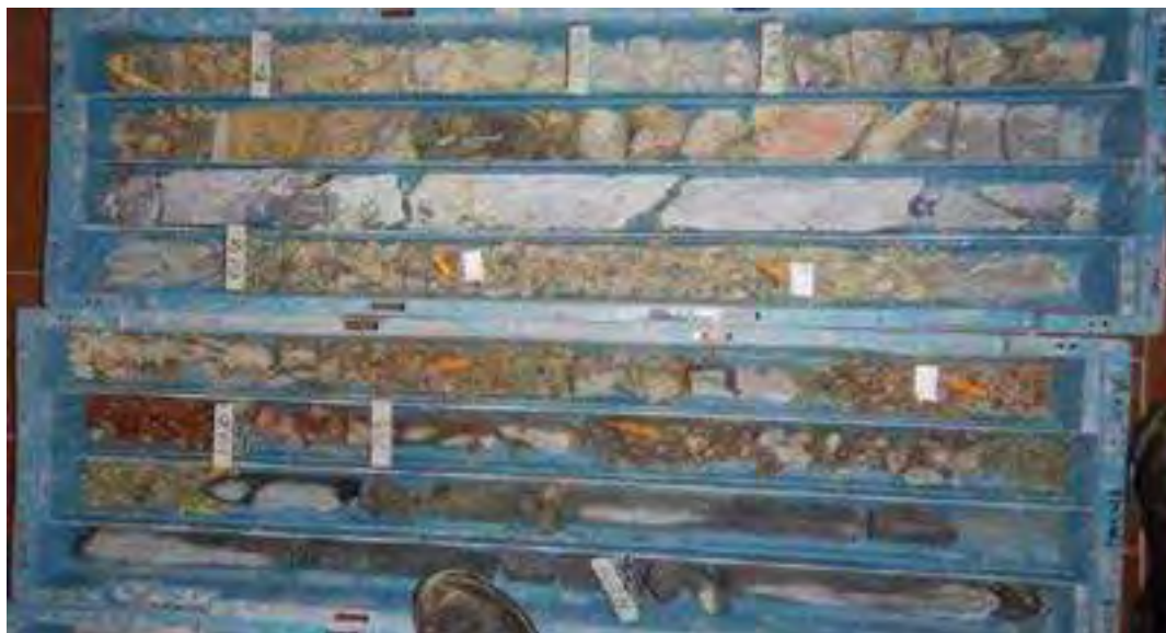
Photo 4.10.2: FWMISED 2017 Core Showing Reaction During Storage and Low-pH Values
