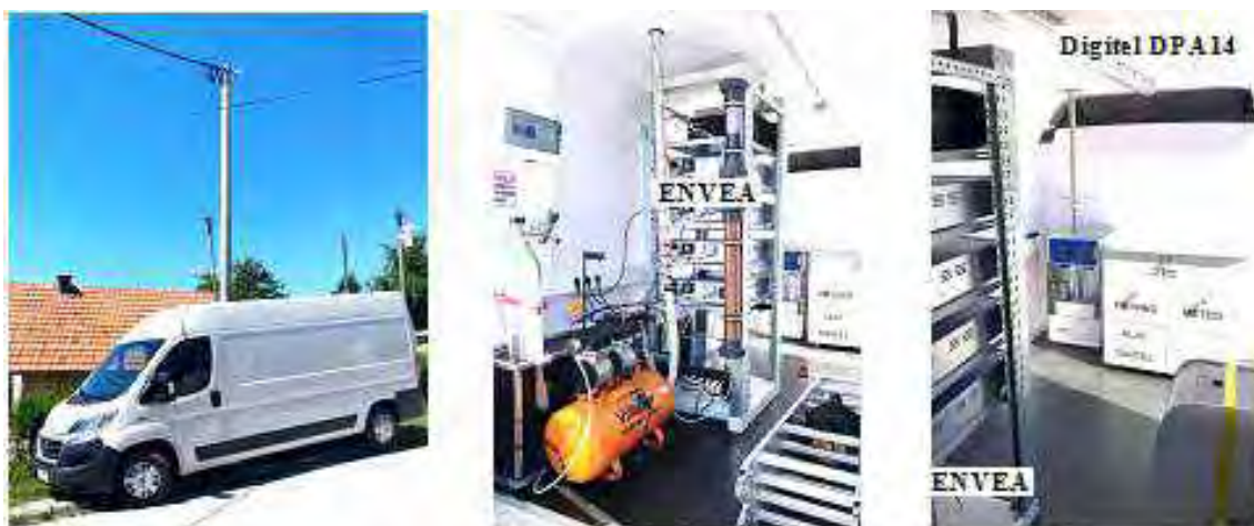
Figure 4.7.1: Mobile Air Quality Monitoring Station
