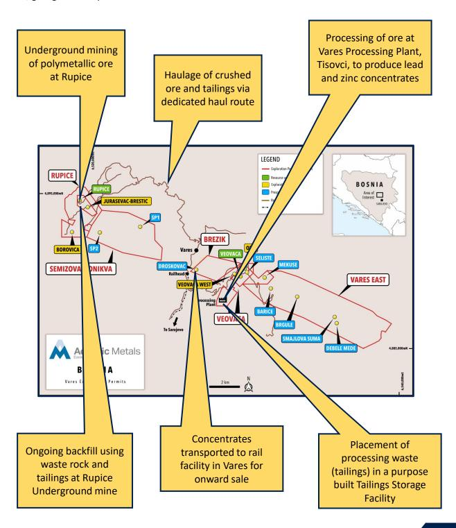
The overall footprint of the Project is 72ha, comprising 28.5ha at the Rupice Mine; 4.5ha for the processing plant; 11ha for the tailings storage facility; and a 28ha haul road corridor. Of the total development, 4.5ha is land previously used for mining and approximately 9ha consists of existing road.
