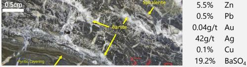
Barite occurs as sparry accumulations that comprise veins, fracture infill, and as acicular overgrowth of sedimentary matrix material, including layers comprised of fine-grained pyrite.
