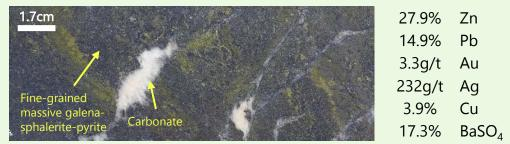
Example of post-mineralisation carbonate veining (from BR-5-18<sup>3</sup>), which appear to be the last structures developed at Rupice
