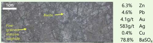
Mineralisation (from BR-3-18<sup>2</sup>) presents as lenticular zones of sulphide layers, clasts, and foliated masses. Sulphide is present as the dark material occurring with white barite.
