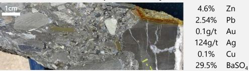
The principal host to mineralisation is a poorly sorted polymict breccia, showing variation in clast type and size. Mineralisation is present in both matrix and clasts.
