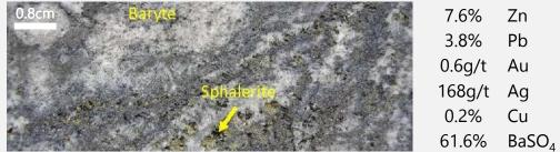
Sphalerite appears spatially close to barite but, in detail, overprints the barite.
