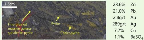
Also, from BR-5-18<sup>3</sup>, zones of massive pyrite are cut by sphalerite-chalcopyrite veins and lenses. Overprinting relationships between massive pyrite and other sulphides consistently indicate the pyrite formed prior to base metals.
